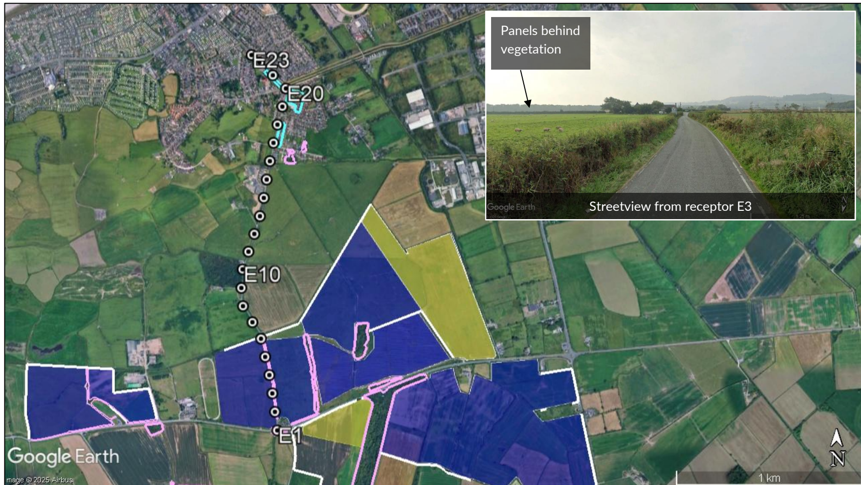
Figure 26 Screening for road receptors E2 to E23, with Streetview from receptor E3
