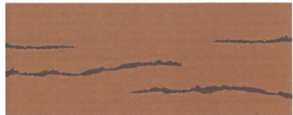
Figure 7. Natural pans – often very hard bands of soil particles cemented together by iron and manganese
