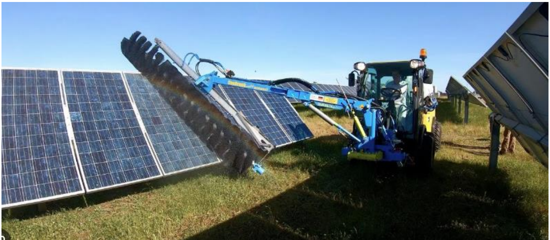
Photo 30: Cleaning of Solar Arrays
