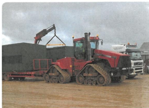
Case Steiger Quadtrac used to deliver inverters and other heavy equipment to site under soft ground conditions (photo courtesy of British Solar Renewables)
